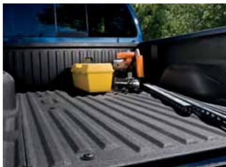
**Shields your investment.** Go for the Tough Bed® factory-installed spray-in bedliner,<sup>2</sup> and an industrial-grade synthetic lining will be applied with a precision high-pressure automated sprayer to help ensure a smooth, even and durable coat.
