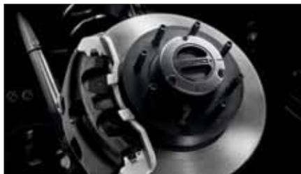
**Stops more confidently – new larger brakes.** The 2013 Super Duty features a 16% increase in the rotor swept area up front and a 15% increase in the rear, helping to provide a more confident brake feel than on previous models.
