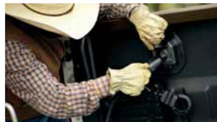
**Makes connecting easy.** Plug in your trailer wiring while standing upright with our class-exclusive in-bed 7-pin connector, part of the 5th-Wheel/Gooseneck Trailer Tow Prep Package<sup>1</sup>.
