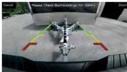
**Helps you line it up.** With the rear view camera<sup>1</sup>, you just shift into Reverse and a full-color image of what's behind the truck is displayed in your rearview mirror or on the 8" MyFord Touch<sup>®</sup> screen (shown).
