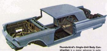
ventional chassis frame. Floor pan, frame, body side panels, front and rear fenders, roof panel, roof cross braces—all are welded together into one durable integral unit of double-walled sculptured steel. Result: the strongest body it has ever been possible to build!
