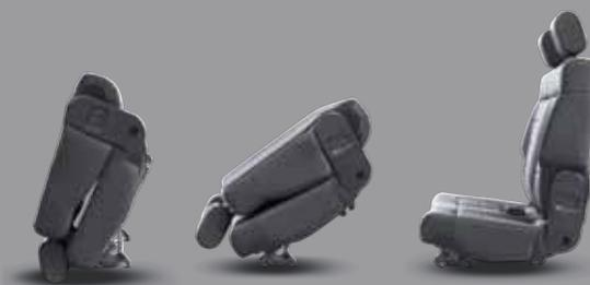
**STANDARD FOLD AND TUMBLE REAR BENCH SEAT.** Make more room for people, cargo, or pets. Easy to rearrange, these seats easily tumble forward and are found on all Wrangler two-door models. Wrangler four-door models come standard with a split-folding rear seat.
