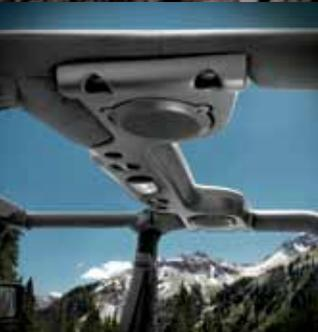
**SOUND POSSIBILITIES.** Radios with MP3 audio input jacks and six-speaker audio system are standard. There are two tweeters and four 6.5-inch speakers (two in the overhead sound bar). Available is a premium sound system that includes six Infinity® speakers and an 8-inch subwoofer with a 368-watt amplifier.
