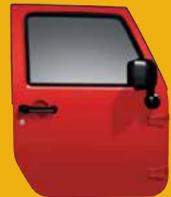
**FULL-FRAMED DOORS.** Removable<sup>SM\*</sup> with roll-up windows and available power windows and door locks. Map pockets with mesh net to ensure wash-out capability. Aluminum-forged hinges are used on both Wrangler and Wrangler Unlimited. (Standard on all models.)
