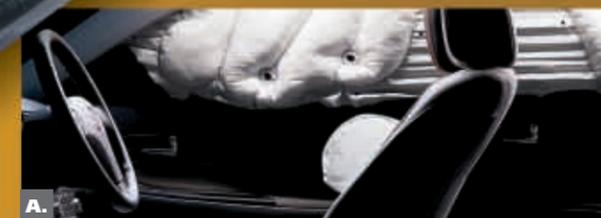
**A. PROTECTIVE MEASURES.** Dual two-stage front air bags\* that help match inflation speed to an impact's severity, plus whiplash-reducing front-seat head restraints and 3-point safety belts for all five occupants are standard on all MAZDA6 models. Side air curtains (with coverage for front and rear seats) and front seat side-impact air bags\* are standard on most MAZDA6 models.
