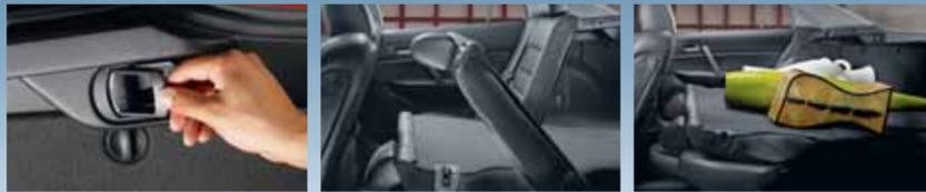
Pulling one or both of the two remote control levers inside the liftgate automatically activates the 60/40 split fold-down rear seatback's handy "fold-flat" feature, moves the rear seat bottom forward and creates a virtually flat load floor. With its rear seatback in the upright position, the MAZDA6 5-Door offers seating for three adults plus a surprising 22.1 cu ft of cargo space behind the seatback.\*
