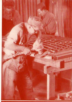
In Fisher composite body construction . . . steel reinforces wood . . . and wood reinforces steel . . . to assure maximum safety, comfort and durability.
