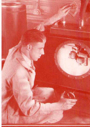
Carburetor efficiency . . . a vital factor of economy . . . is determined with scientific precision by testing performance in a mercury-sealed compartment.
