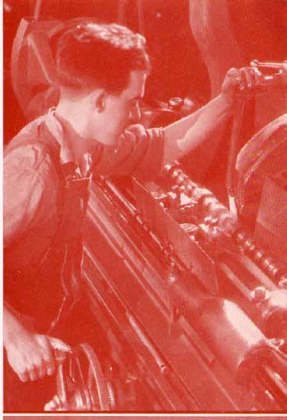
The mirror-like smoothness to which all cam and bearing surfaces are ground is among the important factors contributing to quiet operation.
