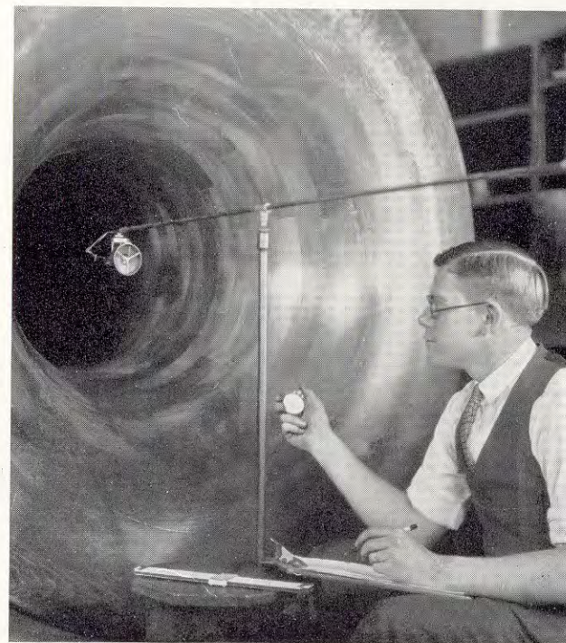
By means of this wind tunnel the cooling efficiency of radiators and fans is accurately established.
