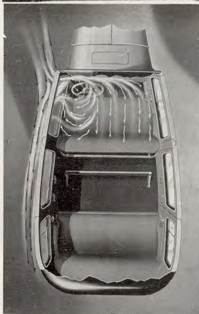
Driver's window down, ventilator open. Arrows show how air flows across windshield, preventing clouding in stormy weather
