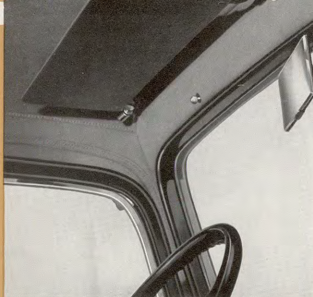
The interior sun visor is quickly adjustable from both front and side and can be tilted to any desired angle to protect the driver's eyes.
