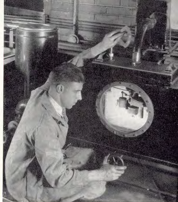
Carburetor efficiency is determined with scientific accuracy in a mercury-sealed compartment.
