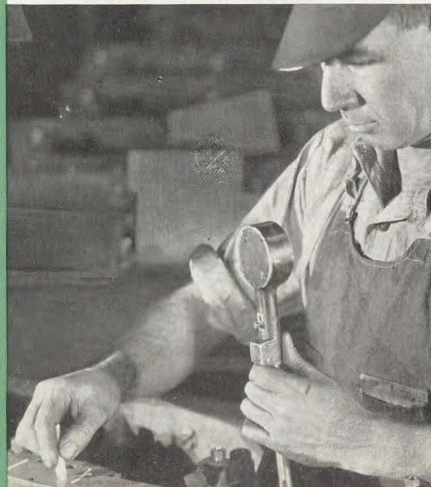
All cylinder barrels are triple-gauged for size and shape to insure accuracy, uniformity and long life.
