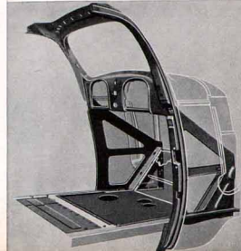
ALL-STEEL BOX SECTION WIND-SHIELD POST . . . The entire section of the front part of the body is given super-strength and super-rigidity by a steel-reinforced-by-steel construction.
