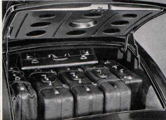
REAR COMPARTMENT, BUSINESS COUPE . . . Unusually generous accommodations for luggage and salesmen's samples are provided in this business coupe. The rear deck of this business coupe is 46 inches long, 45 inches wide, and has a maximum height of 26 inches. Note the number of suit cases it is capable of carrying.
