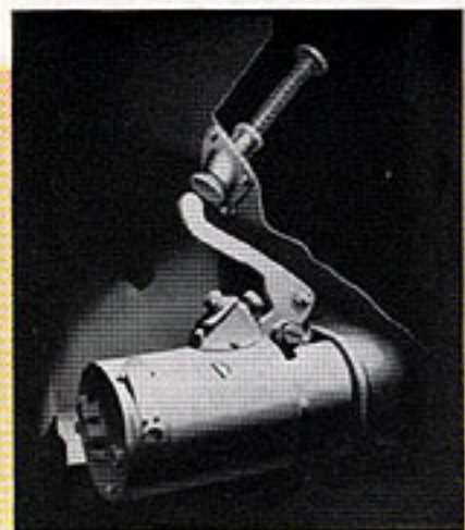
Positive Shift Starter: Starter gear meshes positively with engine flywheel before the sturdy starter begins cranking. Plunger-type starter pedal is isolated from the engine. (Above left)
