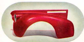
Front fender, lamp housing and hood side of the Buick Roadmaster are stamped from a single piece of sheet metal—a much simpler and stronger construction.
