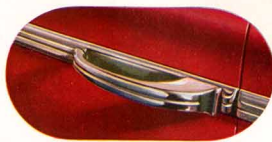
Exterior door handles, mounted through the body belt moulding, curve back to form a safety loop. Large and heavy, they give a firm grip for opening the door.
