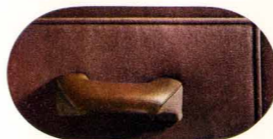
Armrests, shaped to serve as door pulls, are conveniently placed on both front doors. They are trimmed with leather on top to prevent wear.
