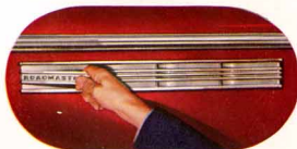
This decorative chrome-and-silver element serves as a latch for the hood cover. The hood is released when the bar is swung out as illustrated in the picture.
