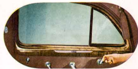
Ventipanes built into rear doors give rear seat passengers complete and individual control over ventilation.
