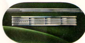
Lou-locks having wider-spaced chromium bars carry the Series name and serve as hood latches. The space between bars has the appearance of sand-blasted silver.
