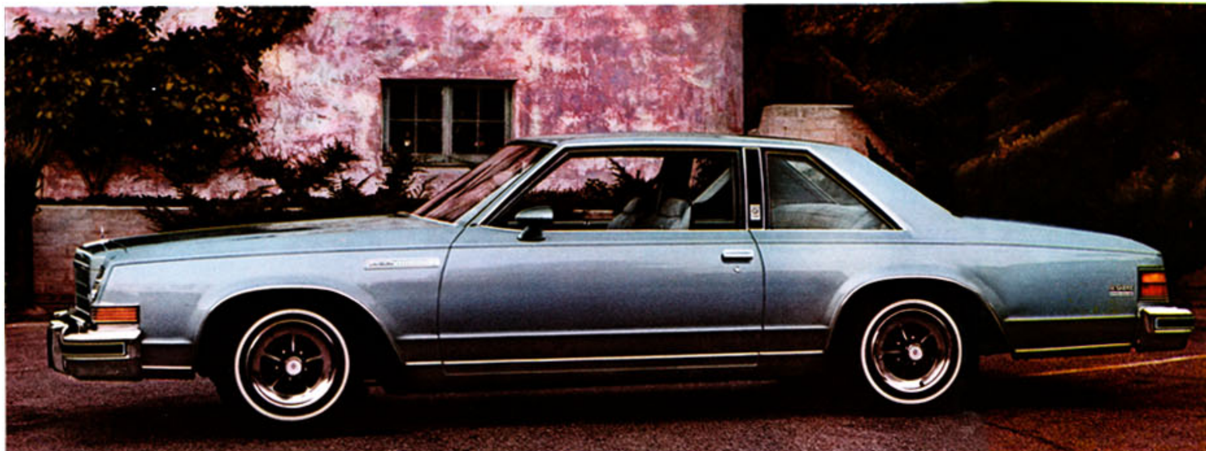
LeSabre Sport Coupe. Engineered for the enthusiast with a special ride-and-handling package and a 3.8 litre (231 CID), turbocharged V-6.
