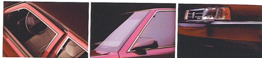
From left to right: wrap-over doors and semi-flush side windows provide structural integrity and reduce wind resistance; a low-profile windshield and aero-style side mirrors enhance airflow and contribute to Premier's sleek, streamlined appearance; a front air dam helps to reduce drag and facilitates better engine cooling at highway speeds.
