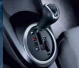
*The available dual-mode transmission with SHIFTRONIC™ offers fully automatic or manual sport shifting.*
