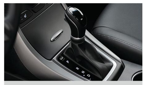
SHIFTRONIC WITH ACTIVE ECO SYSTEM Elantra Limited comes standard with a 6-speed SHIFTRONIC automatic transmission that makes the most of the engine's silky-smooth 145 horsepower. It features a locking torque converter for better fuel economy at freeway speeds, and an Active ECO System that modifies engine and transmission controls at the press of a button for further fuel economy efficiencies.
