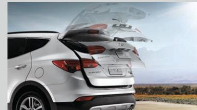
**HANDS-FREE SMART LIFTGATE** How smart is this available feature? Stand within three feet of the vehicle's rear liftgate with the key in your pocket or purse for more than three seconds, and it opens automatically. No kicking your feet to activate it. You can stop the liftgate at various heights, too.
