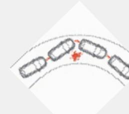
The computer sensors of the Vehicle Dynamics Control (VDC) system continually monitor driving conditions to detect and help correct unintended deviations in the vehicle's trajectory and help set you back on the correct path.
