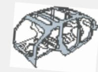
Engineered for exceptional strength to help maintain the integrity of the cabin structure, the innovative Subaru ring-shaped reinforcements around the passenger compartment also help dissipate crash-impact energy away from occupants.
