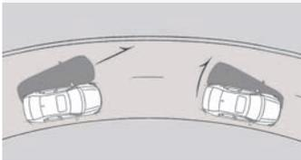
**VEHICLE STABILITY ASSIST™ (VSA®)** THIS SYSTEM CAN BRAKE INDIVIDUAL WHEELS AND/OR REDUCE ENGINE POWER IN THE EVENT OF UNDERSTEER OR OVERSTEER TO HELP KEEP YOU ON YOUR INTENDED PATH. A TRACTION-CONTROL FUNCTION HELPS PREVENT WHEELSPIN DURING ACCELERATION.
