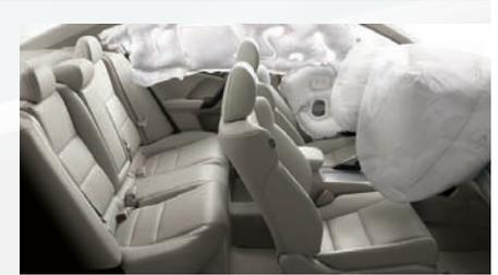
**ADVANCED AIRBAG SYSTEM** DUAL-STAGE, DUAL-THRESHOLD FRONT AIRBAGS, FRONT SIDE AIRBAGS AND SIDE CURTAIN AIRBAGS ARE ONLY PART OF ACURA'S COMPREHENSIVE APPROACH TO PASSIVE SAFETY. AN OCCUPANT POSITION DETECTION SYSTEM (OPDS) IS DESIGNED TO PREVENT DEPLOYMENT OF THE FRONT PASSENGER'S SIDE AIRBAG IF A SMALL-STATURED OR AN OUT-OF-POSITION FRONT PASSENGER LEANS INTO THE AIRBAG'S DEPLOYMENT PATH.\*
