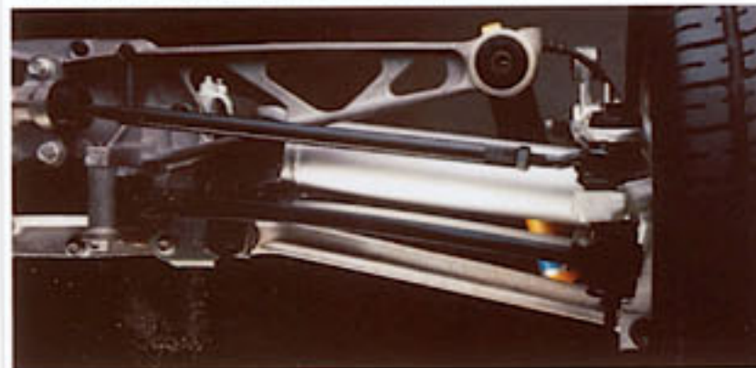
Corvette's sophisticated fully independent suspension is an important reason why this car is so much fun to drive. Components include forged aluminum control arms, transverse springs and stabilizer bars and a 5-link independent rear design that helps maximize tire patch contact with the road surface.
