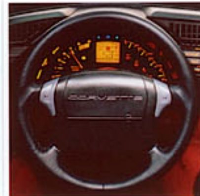
The new-for-1990 Supplemental Inflatable Restraint system (air bag) is located in the hub of the steering wheel. The SIR is designed to provide added protection in the event your Corvette is involved in a moderate to severe frontal collision. For maximum protection in frontal and all other collisions, both driver and passenger should be properly restrained with safety belts.
