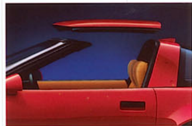
Corvette Coupe features a standard removable roof panel (one-piece with no center T-bar).
