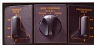
Selective Ride Control's console-mounted switch allows you to select the ride firmness you desire (Touring, Sport or Performance).
