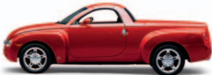
The retractable roof consists of two stamped steel panels and a deep-tinted fixed backglass. Triple weather seals provide the added protection needed for the Canadian climate.
