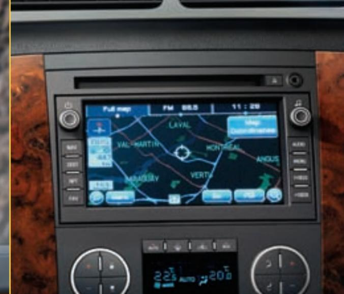
Enhance your sense of direction. The touch-screen DVD navigation system\* features a large full-colour touch-screen monitor and voice recognition that responds to as many as 26 different commands. The system enables you to choose between different routes and provides step-by-step directions to your selected destination. It also alerts you if you stray from your course. It even develops a new, preferred route if you make a wrong turn. Available on Extended and Crew Cab LT and LTZ models.
