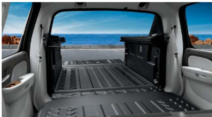
4 To complete the transformation, remove the rear window and three-piece cargo cover and lower the tailgate to transport items such as a small ATV.
