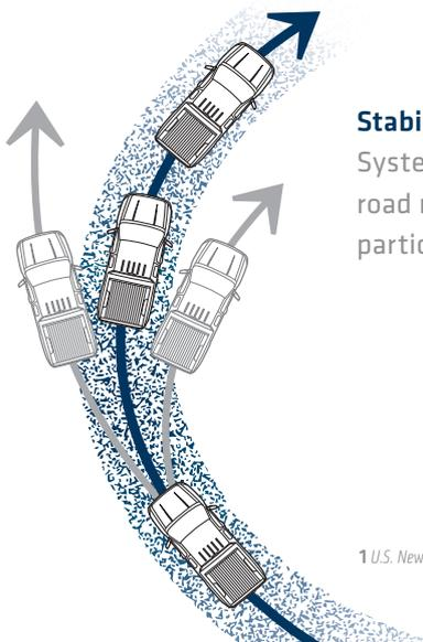
**StabiliTrak.** The StabiliTrak Electronic Stability Control System with Traction Control helps you avoid what the road might throw at you by improving vehicle stability, particularly during emergency maneuvers.
