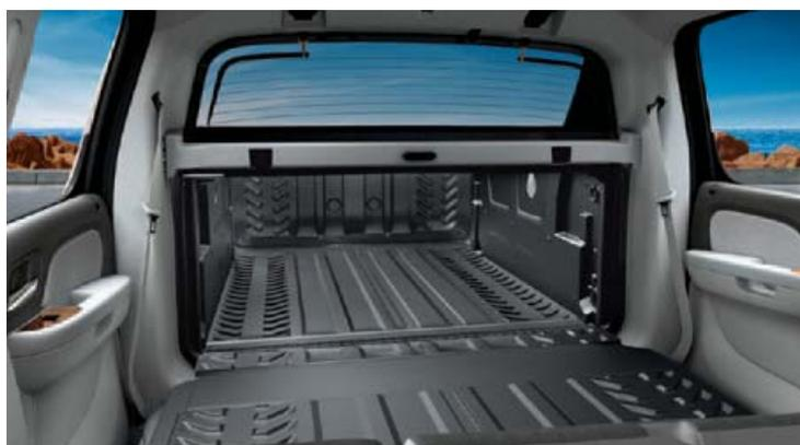
3 To utilize the full length of the cargo box, just lower the Midgate for a completely secured cargo area (when the three-piece cargo cover and rear window are in place).
