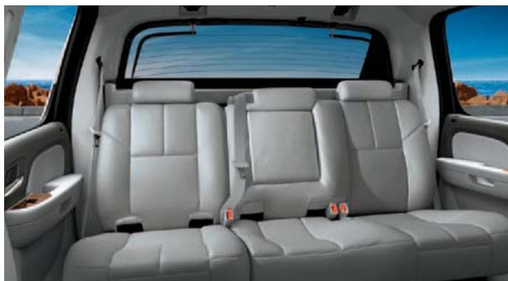
1 With the 60/40 split-folding rear-bench seatback and Midgate upright, Avalanche can be configured as a five- or six-passenger<sup>3</sup> SUV.
