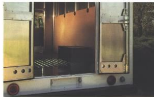
► Standard dual rear doors provide a 38" wide opening for loading.
