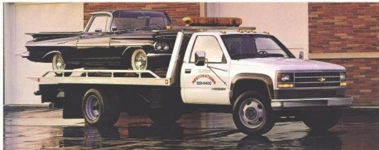
▲ C3500 HD straight-rail Chassis-Cab in Frost White with car retriever body from independent supplier.
