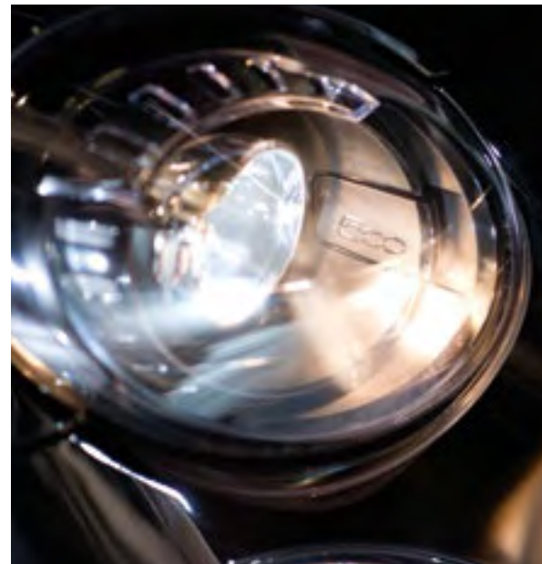
Bi-halogen projector headlamps provide more controlled illumination for increased visibility.
