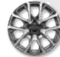
18-INCH MACHINED ALUMINUM WITH MATTE CHROME PAINTED SHADOW EFFECT AND GLOSS-BLACK CENTER Standard on 500X Trekking Plus
