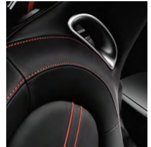
High-back bucket seats incorporate a racing harness pass-through and firm side bolsters.
