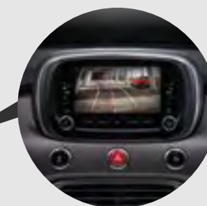
PARKVIEW REAR BACK-UP CAMERA 7 Image is displayed on a color touchscreen when the vehicle is in Reverse. Contains dynamic grid lines to aid the driver.
