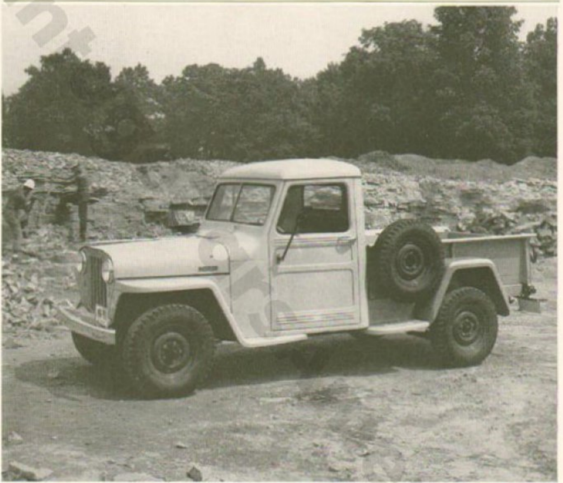
The Four-Wheel-Drive Truck, with a rated one-ton payload, meets the needs of truck users who want two-wheel drive economy on hard roads, plus selective four-wheel drive for extra tractive power
