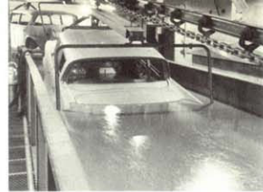
Full-Dip Rustproofing: Like all Ramblers, the entire body structure is dipped in a full rustproofing bath to prevent rusting from inside out.
