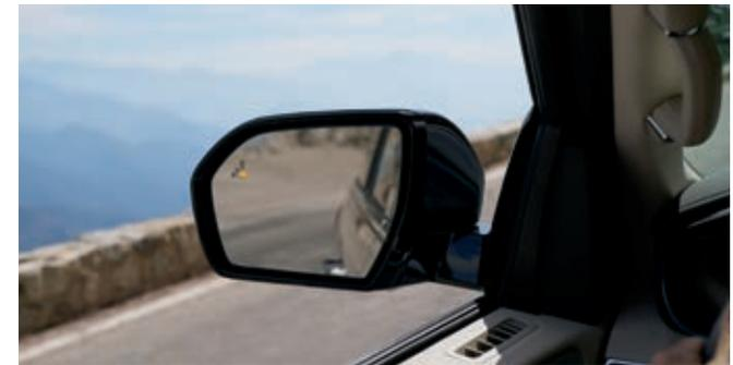
**BLIS® (BLIND SPOT INFORMATION SYSTEM) WITH TRAILER COVERAGE<sup>1</sup>** – Some vehicles may be out of your line of sight, but they can be detected by this technology. It warns you if it detects a vehicle in your blind spots while driving forward, or approaching from the sides while in Reverse. The range of coverage can also be extended to include a conventional trailer, once it's been programmed into the system.
