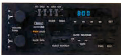
▲ Optional ETR AM stereo 1/FM stereo radio with premium dual rear speakers, seek and scan, graphic equalizer and digital clock, plus stereo cassette tape player with search and repeat.
