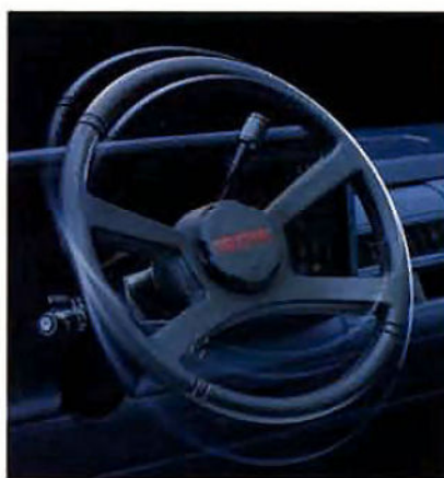
◀ Optional Driver Convenience Group consists of Comfortilt steering wheel and electronic speed control. Comfortilt makes getting in and out of the driver's seat easy and also gives the driver a just-right adjustment for short trips and long ones. (Shown with Silverado Sport steering wheel.)
