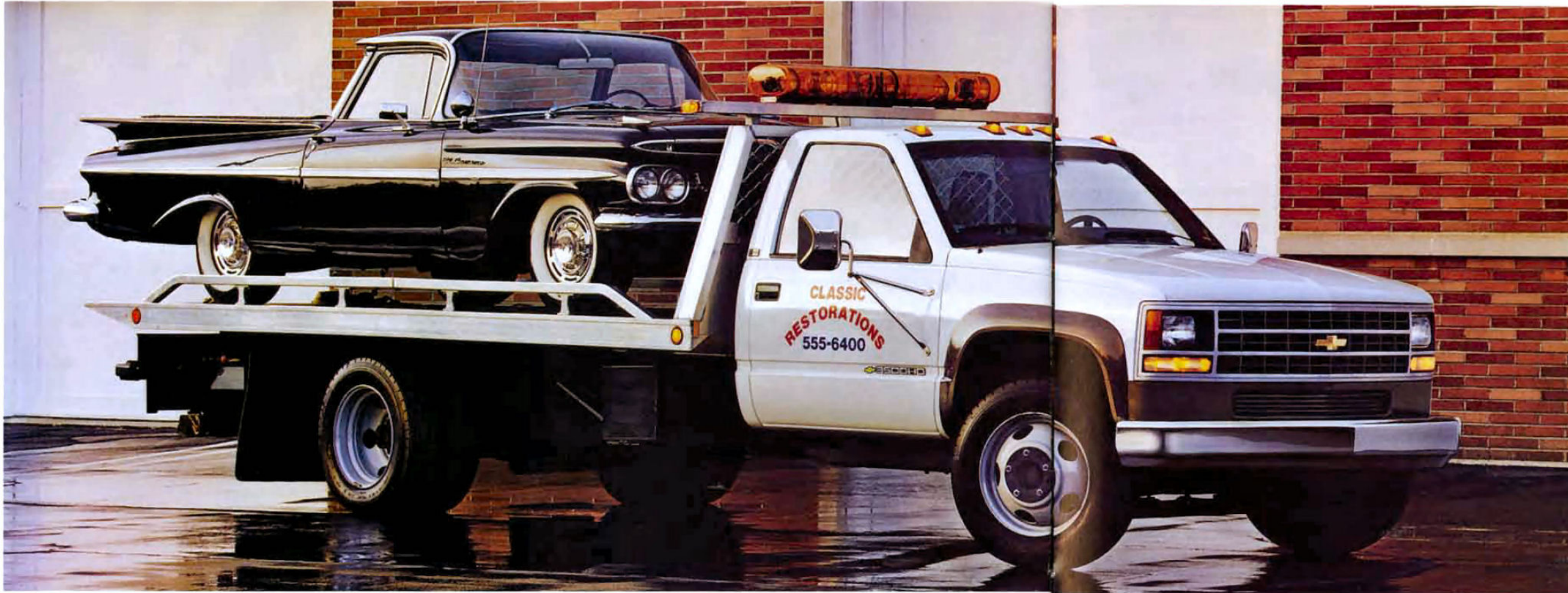
▲ New C3500 HD Chassis-Cab in Summit White with straight rails for easy mounting of special bodies. Shown here with retriever body from independent supplier.
