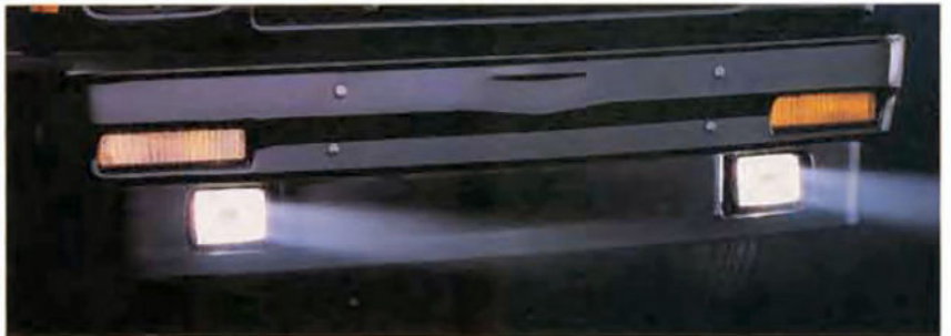
▲ Optional fog lamps can be ordered for standard air dam on 2WD models. Standard air dam on 4x4 models includes tow hooks.
