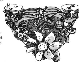
Power surges through long aluminum tube intake manifolds which use outside air to pack a maximum of fuel mixture into the carburetion system. Two, four-barrel carburetors deliver the charge to special high-performance plugs. The "J's" healthy breathing is further aided by two special competition-type air cleaners.
