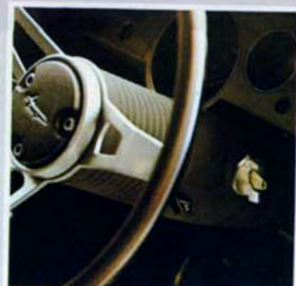
Anti-theft, column-mounted ignition switch.
