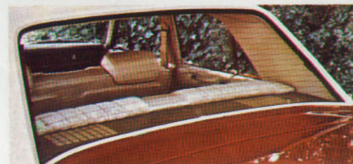
Electric rear window defroster.
