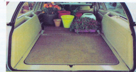
Carpeted rear cargo deck has 86.8 cu. ft. of load space for 4' x 8' materials with doorgate closed.
