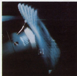
Tilt steering column adjusts to 6 positions to suit any driver.
