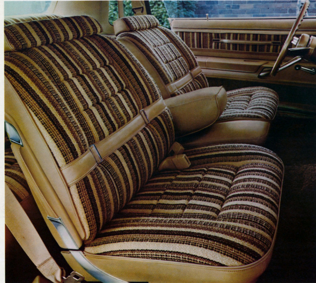
Optional 60/40 Boca Raton split-bench seat in rich woven cloth and grained vinyl with center armrest and dual reclining seat-backs.
