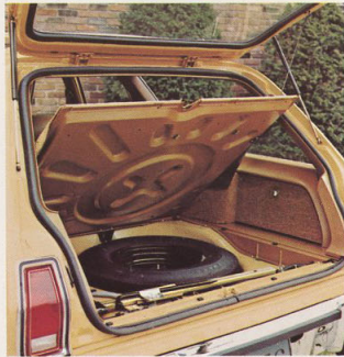
Standard spare tire well is recessed below cargo area. Lockable side storage compartments standard on Premier.
