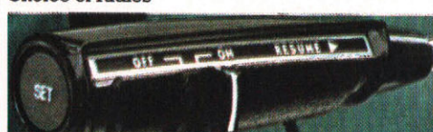
Automatic speed control
