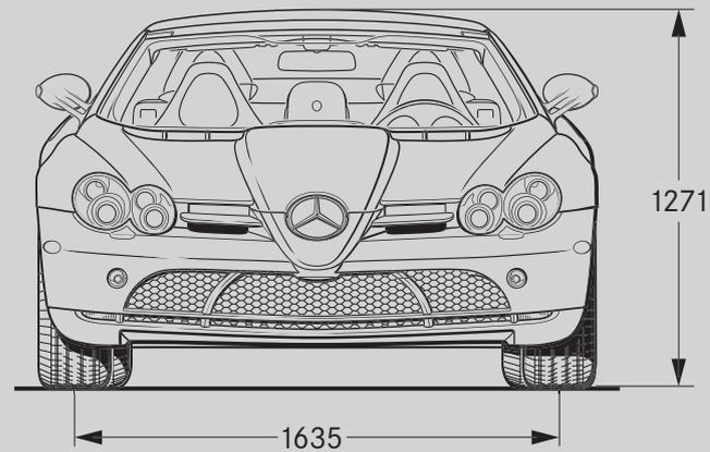
All measurements are in millimetres. The dimensions shown are mean values and apply to standard-specification, unladen vehicles.
