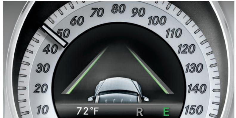
**Multilane multitasker.** Optional Lane Keeping Assist uses a camera to monitor the vehicle's position in relation to visible lane markings. If you start to drift out of your lane without signaling, it can alert you by vibrating the steering wheel. It's also available with advanced active technology that can gently apply the brakes to individual wheels, to help draw the vehicle back into its original lane if you disregard the alerts.<sup>7</sup>
