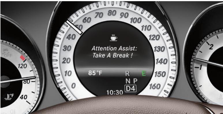
**A watchful eye when's it time for a rest.** ATTENTION ASSIST<sup>®</sup> is a Mercedes-Benz innovation that can alert you if it detects signs of drowsiness on long drives. It measures more than 70 variables, starting in the first minutes of a drive, to establish a pattern. By continually monitoring a variety of driving behaviors along your trip, it can offer a warning tone and encourage taking a rest if it senses you're getting drowsy.<sup>7</sup>
