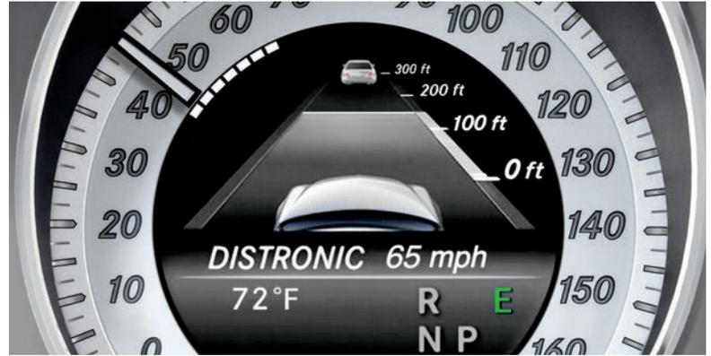
**Cruise control that stops and goes.** DISTRONIC PLUS<sup>®</sup> adaptive cruise control uses radar to adapt your set speed in response to the flow of traffic ahead. It can slow the vehicle automatically—or brake to a stop—then resume with a tap.<sup>7</sup> Even if you're not using cruise control, PRE-SAFE<sup>®</sup> Brake can alert you to stopped traffic, and automatically apply up to 100% braking force to help prevent or reduce the severity of an impact.<sup>8</sup>
