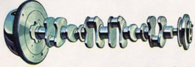
Sturdy backbone of this power-plant is the massive 7-bearing Nash crankshaft, 100% counterbalanced—its mate found only in one other car in the world, Rolls Royce.
