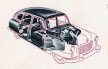
AIRFLYTE CONSTRUCTION—the greatest single advance in motor car construction in 40 years... the key to safety, comfort, economy and performance you have never known before in an automobile. With Airflyte Construction—exclusive to Nash—body and frame are one integral unit, eliminating noise-making joints, bolts and nuts.
