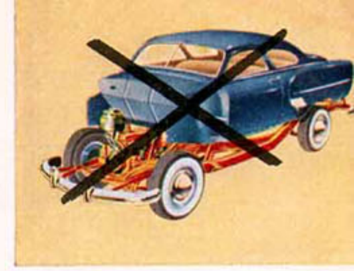
In cars built the ordinary way, a separate body is bolted on a heavy frame. There is less protection for passengers, the car has less strength and rigidity and body tends to squeak and rattle.
