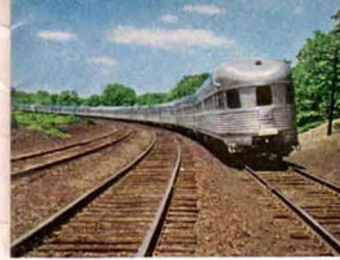
The "Streamliner" revolutionized travel because its integral-braced structure rode better, proved safer, than the old-type coach which was bolted on a heavy, hard-riding platform.
