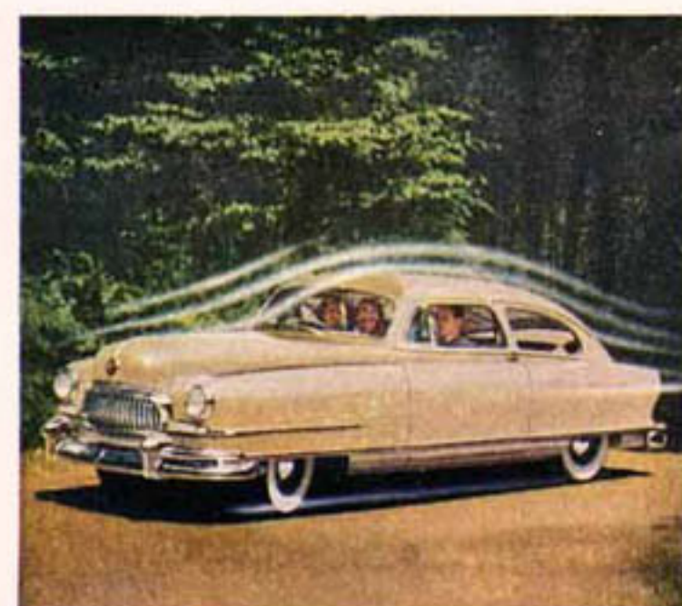
Best in aerodynamic efficiency. (1) Sleek, clean front and curved windshield slip through the air. (2) Sleek "tear-drop" shape reduces air drag vacuum at rear. (3) Enclosed wheels eliminate worst air traps, reduce wind-wander. (4) Airflyte Construction reduces air turbulence beneath.
