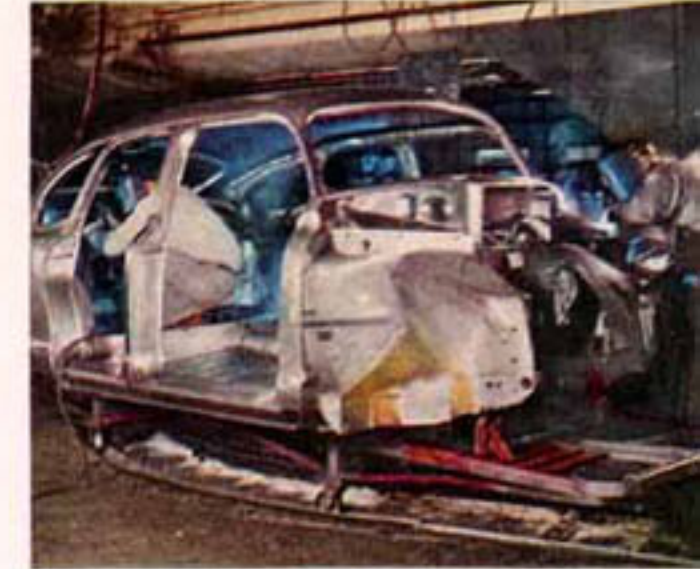
In Nash, 8000 electric welds eliminate noise-making joints — give you lifetime freedom from body squeaks and rattles. The weakest structural parts of other cars — bolts and flanges fitting body to frame — are eliminated by Airflyte Construction.
