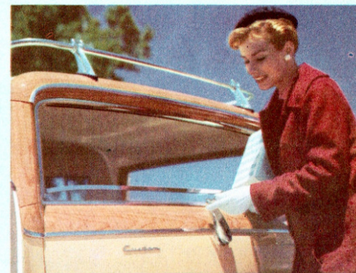
ROLL-DOWN REAR WINDOW—on all 1958 station wagons disappears into tail-gate. The one-piece cargo door eliminates upper hinges... gives more loading room.
