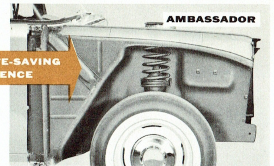
AMBASSADOR See how big box-sections extend forward from the massive box-girder cowl on each side of the Ambassador engine to absorb impact.
