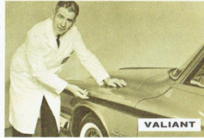
Valiant's sculptured side body metal, like the Falcon's, is expensive to repair. Rambler's smooth panels cost much less to repair.
