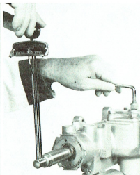
Adjusting Pitman Shaft end play
