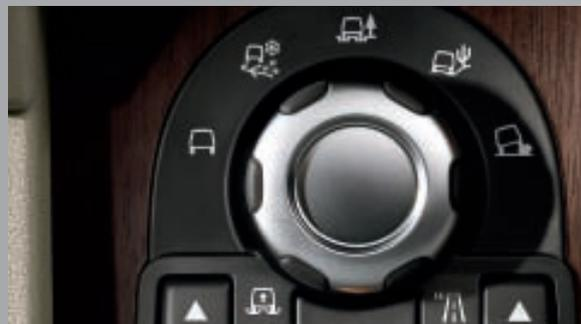
**THE AWARD WINNING TERRAIN RESPONSE® SYSTEM** optimizes the vehicle set-up for virtually all on-road or off-road driving situations, with five different settings to suit different terrains such as grass/gravel/snow, mud and ruts, sand and rock crawl.
