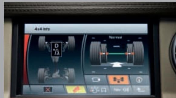
**AIR SUSPENSION.** Four-corner independent Air Suspension with variable ride height and electronic cross-linking for a constant level ride height. Ride height can be raised up 2.2 inches/55mm to clear obstacles or lowered by 1.9 inches/50mm for easy access and loading from standard ride height.
