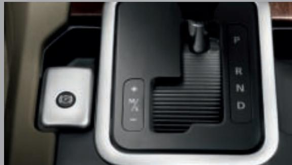
**ELECTRIC PARKING BRAKE (EPB).** A lever is located next to the gear selector to electrically apply and release the parking brakes on the rear wheels. A simple pull of the lever applies the brake manually and a press releases it. The parking brake will also release automatically upon driving away.
