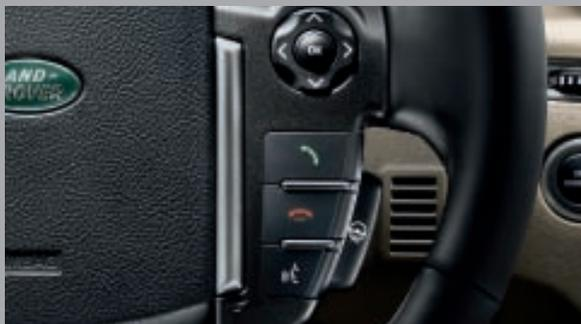
**STEERING WHEEL CONTROLS.** Steering wheel with ergonomically designed switch layout for driver information and remote audio controls. Cruise control is standard while telephone and heated steering wheel controls are optional and dependant on the vehicle derivative.
