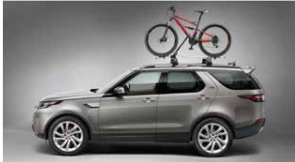
**Roof Mounted Bike Carrier – Wheel Mounted\***
