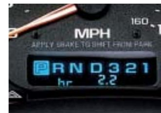
**ENGINE HOUR METER.** A standard engine hour meter indicates how long your engine has been in use. It's a feature that you'll appreciate having, especially if your truck spends a lot of time idling.
