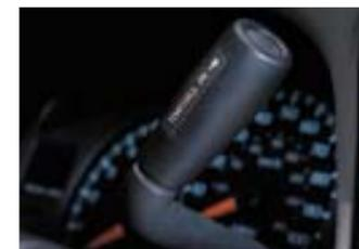
**TOW/HAUL MODE.** Tow/Haul mode, when activated, enhances trailering by reprogramming the optional automatic transmission shift schedule when you're transporting heavy loads.
