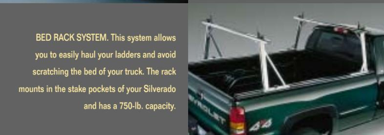
BED RACK SYSTEM. This system allows you to easily haul your ladders and avoid scratching the bed of your truck. The rack mounts in the stake pockets of your Silverado and has a 750-lb. capacity.
