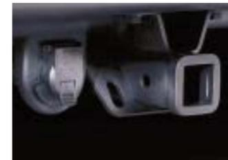
**TRAILER-READY.** The trailer-ready design of Silverado features an eight-wire lead along with an available seven-pin connector and weight-distributing hitch (included with the Z82 Heavy-Duty Trailering Package).
