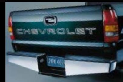
REAR BUMPER. This drop center bumper features a non-skid step pad and a 500-lb. tongue weight.
