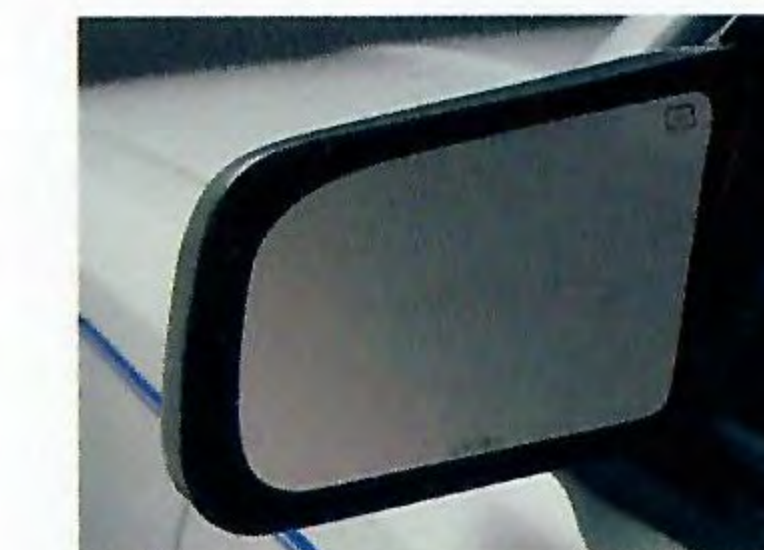
Heated dual power mirrors clear view for driving in ice and snow.
