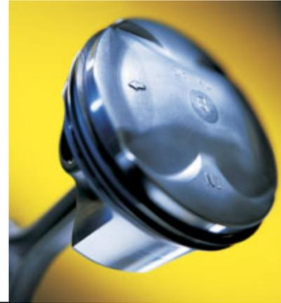
**Smooth operator.** Friction robs power and efficiency, so we took great strides in reducing its effects. The S2000's super-light **forged-alloy pistons** boast a reduced skirt area and tough carburized forged-steel connecting rods. The decreased surface contact between piston and cylinder wall enables greater performance by reducing friction and allowing higher revs.
