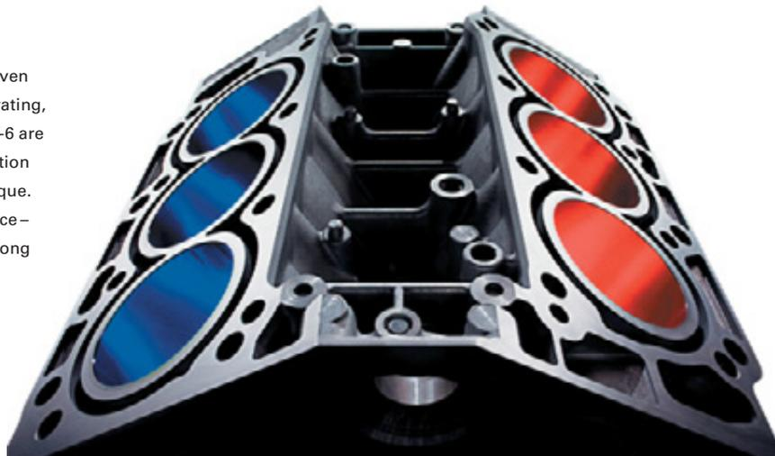
Cruise under light engine loads and VCM deactivates the three rear cylinders. The intake and exhaust valves remain closed, while fuel injection is paused. This can help deliver an EPA highway mileage rating of **28 mpg**.<sup>10,11</sup> Road trippers take note, that's a potential range of nearly **588 miles**.<sup>10†</sup>
