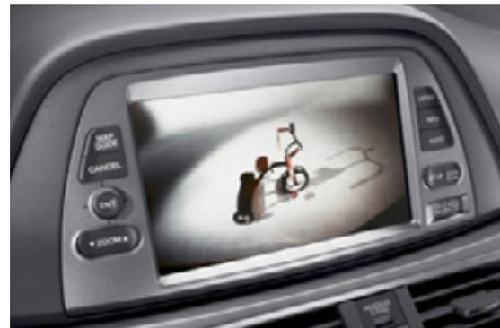
On navigation system-equipped models, the navigation screen doubles as a display for the innovative, full-color rearview camera. When you shift into reverse, the screen offers a clear view of the area immediately behind the vehicle. Parking sensors in Touring models also help keep you more aware of your space.
