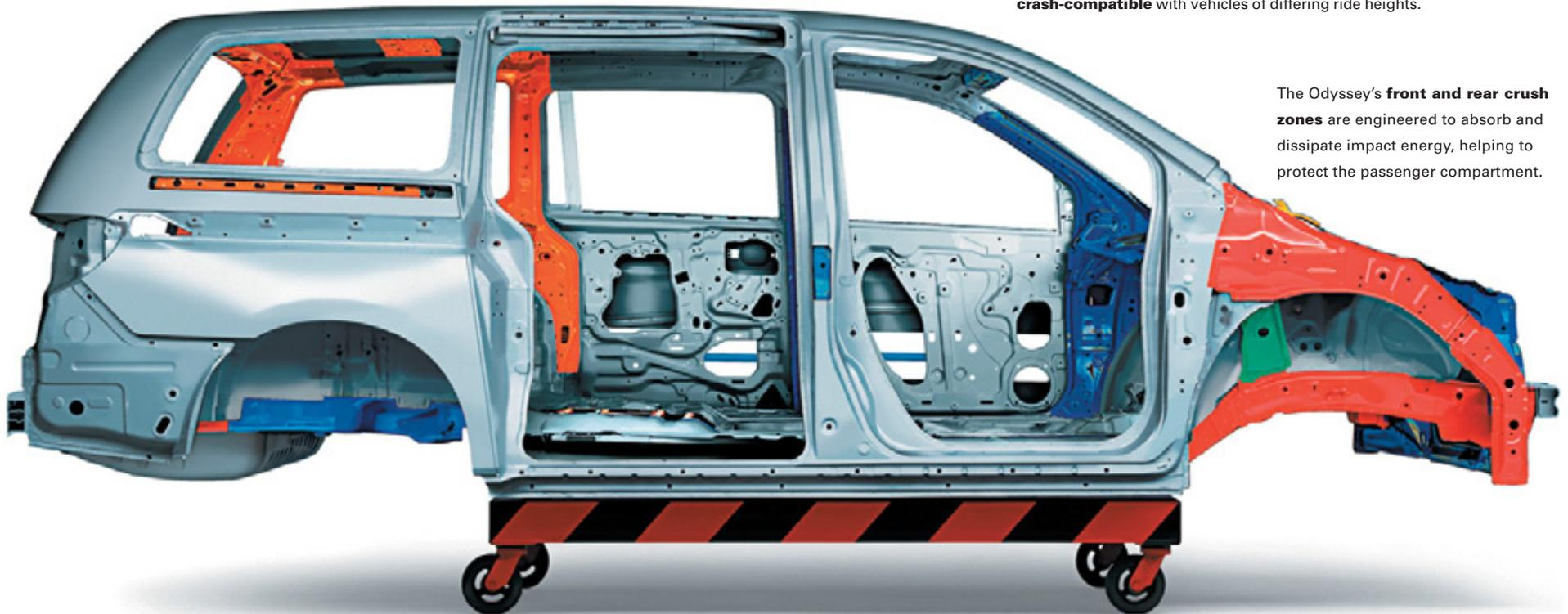
The Odyssey's **front and rear crush zones** are engineered to absorb and dissipate impact energy, helping to protect the passenger compartment.
