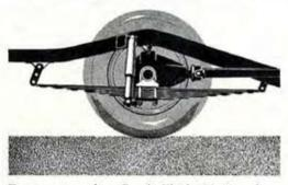
Rear suspension. Semi-elliptical leat springs. The double-acting hydraulic shock absorbers are fitted offset towards the centre of the vehicle to increase stability on bad roads.
