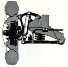
Front suspension. Independent suspension with coil springs and double control arms. Double-acting, hydraulic shock absorbers.
