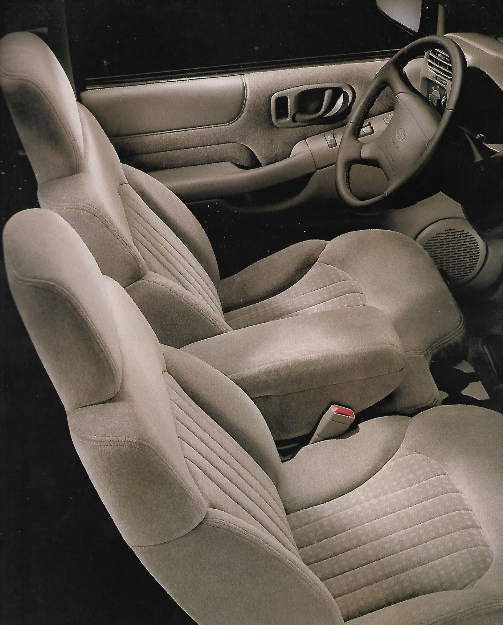
S-10 2WD LS Regular-Cab Deluxe Cloth reclining 60/40 split-bench front seat with center storage armrest in Medium Gray.
