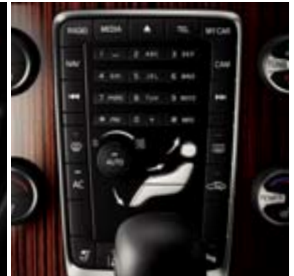
Electronic Climate Control (ECC)
